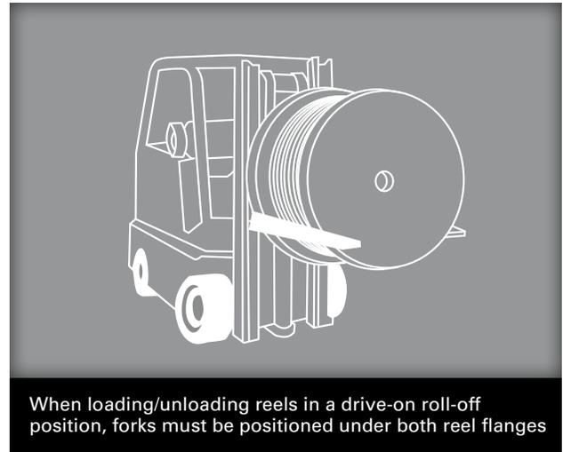
When loading/unloading reels in a drive-on roll-off position, forks must be positioned under both reel flanges
